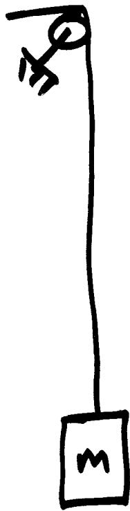
A mine elevator has a cable  $L = 1000 \text{ m}$ , supporting a cab of mass  $4000 \text{ kg}$ .
