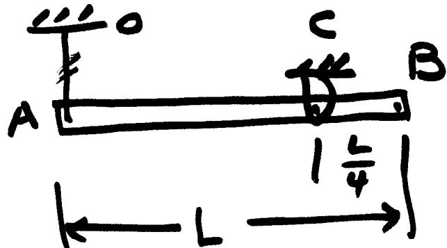
Given: Uniform rod AB, Pinned at C. String OA is Cut.
