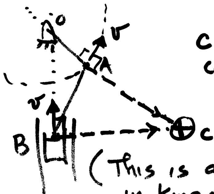
C is I.C. for connecting rod AB.
