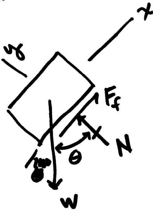
$$\sum F_y = 0 \quad (\text{rectilinear motion along } x \text{ axis}) \Rightarrow a_y = 0$$
