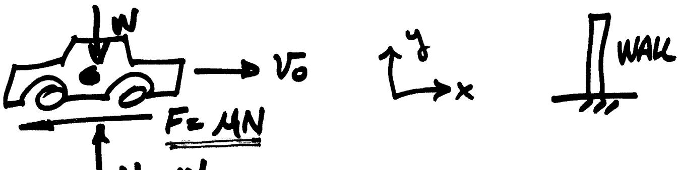
$$W = mg = (3500)(9.81) \text{ kg m/s}^2 = \underline{\underline{34,335 \text{ N}}}$$
